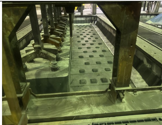
Figure 7. Graphite bed and set anodes
