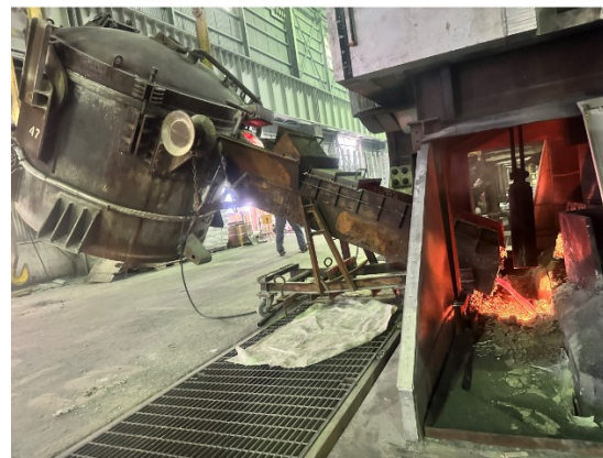
Figure 13. Pilot cells metal pouring.
