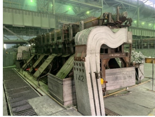
Figure 6. INALUM existing gas preheat arrangement.
