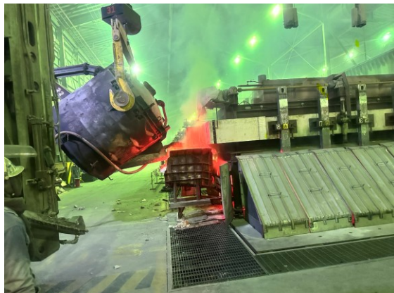
Figure 12. Pilot cells bath-up.
