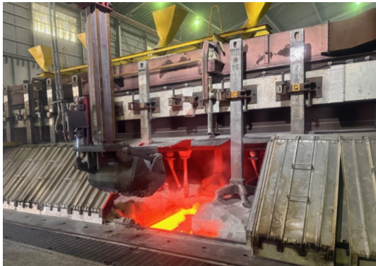
Figure 16. Pilot cells cavity scooping using PTM cavity scoop.
