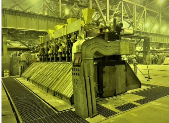
Figure 5. EGA electrical preheat arrangement in pilot cells.
