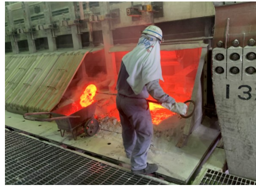
Figure 17. Existing cells manual cavity skimming.
